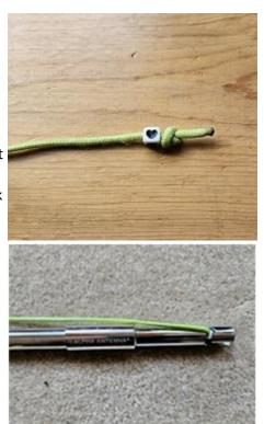
Making the rest of Story String begins with 6 meters. Calculate the length of the whip for the portion of 6 meters you want, set the whip to that length, put it on the tripod and adjust to resonance.
