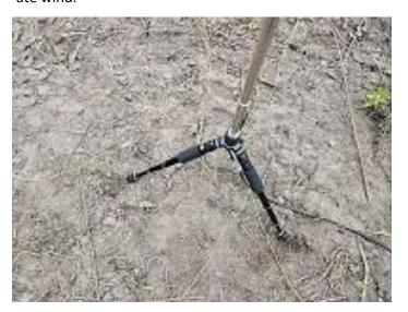
This configuration with the Gabil tripod and a 17 foot collapsible whip antenna is very versatile for operation on the 20 through 6 Meter bands. As an experiment, I extended the whip to its full length and used a tuner to get on 30 meters, it worked.
